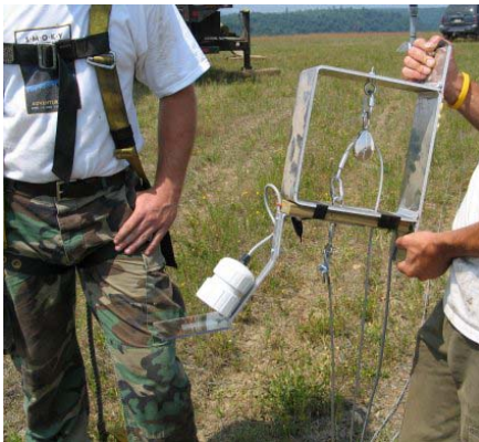
Pulley system for deploying acoustic detector microphones in "bat hats."
